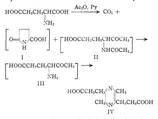
a sirup which after acid hydrolysis (to the salt of III) and basification (with accompanying air oxidation) furnished a small amount of 3,6-dimethylpyrazine-2,5-dipropionic acid (IV).
