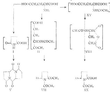
however, is N-acetylated to XV which is internally dehydrated to acetamidoglutaric anhydride, VIII, and this under the conditions of isolation used by us, was rearranged to the acetylpyrrolidone carboxylic acid, IX, a portion of which may also have been formed in the reaction mixture by direct imidic ring-closure of XV.
